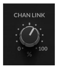
When working with stereo signals, using either 0% or 100% channel linking can cause stereo degradation, depending on the stereo content of the signal.
