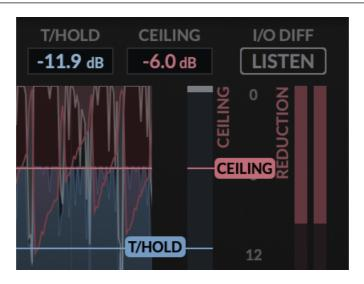
You can also set the **CEILING** and **THRESHOLD** values visually against the incoming signal by using the 'CEILING' and 'T/HOLD' flags/tabs on the Waveform Visualiser. These are also provided as numerical inputs above the graph, so you can always see their value.
