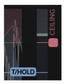
The **CEILING** and **THRESHOLD** parameters can be set by dragging the flags on the graph. Click and drag between the area between the flags to move both parameters at once.
