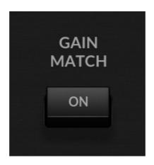
This control automatically adjusts the output to compensate for the **INPUT GAIN** and **THRESHOLD**. This lets you more easily preview the only the perceived effect or character added by limiting, rather than the increase in loudness.
