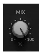
The **MIX** control sets the blend between the 'wet' effected signal and the original 'dry' input signal. A **MIX** control is a rare breed on a limiter, so use it with care - it means that it no longer guaranteed that you signal will not exceed the **CEILING**!
